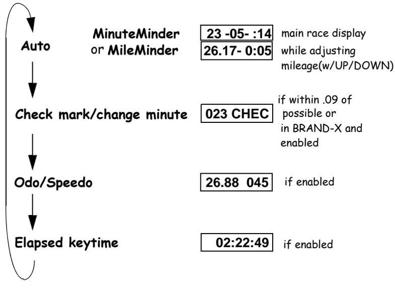
**Race mode displays using UP/DOWN button to select**
