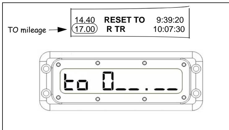
For example, set it to the mileage at the start of the next section (ie. known control mileage). Then as you ride around you will not affect the remaining duration of the gas stop. **Caution!! Don't forget to get out of ICD when you get to the known control!** To exit ICD hold **MAIN** until "ICD OFF" is displayed, then release.
