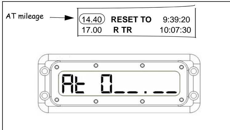
prompting you for the TO mileage of the reset. Enter the TO mileage in the same manner. After entering the last digit the values are stored in memory and the reset function will be displayed again. To continue entering resets hit **MAIN** and repeat.
