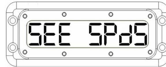
Some letters cannot be displayed in their true form. For instance, K's cannot be formed, so K's will look like capital H's. Therefore H's are always represented in lowercase on the display. Also, an "m" requires two digit fields to represent it in the display. For example, "KEYTIME" on the display looks like:
